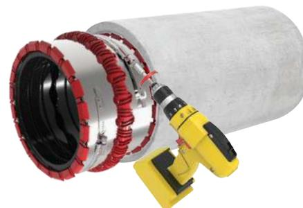
When the coupling ID's are closely matched to the pipe/adaptor OD's, install the coupling onto the ShuvlNose® Adaptor. Take up all slack in coupling with a cordless drill or socket wrench.
