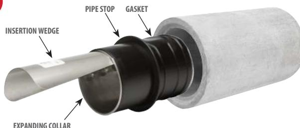
Ensuring the wedge is in line with the top of the pipe, insert the ShuvlNose® Adaptor gasket into the larger pipe up to the pipe stop.
